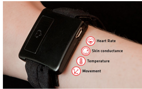
Fig. 2: Empatica E3 wristband – wearable, lightweight, wireless, multi-sensory data acquisition device.
