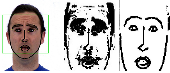
Figure 1: Afraid face in 1a color RGB image, 1b ZCA_{white} representation, and 1c dlib landmark contours representation
